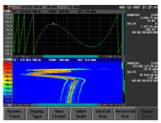
The 3026 captures transition in time, frequency and phase as shown above. The lower portion of the screen displays Amplitude vs. Time (spectrogram), the upper portion displays the phase change during transmitter activation. This example shows this transceiver makes a significant frequency, amplitude and phase shift until it stabilizes.
